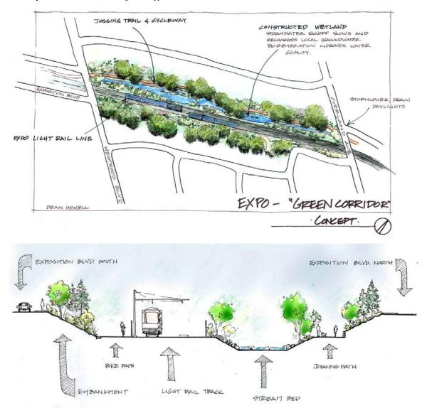
Use of the wide right-of-way for this configuration of light rail tracks in a shallow, soillined trench with short underpass structure may be **no more costly**, and is certainly **much less visually impacting** than a conventional overpass with retained-fill ramps edged with soundwalls. **Water quality funds** may complement transit funds for this.
